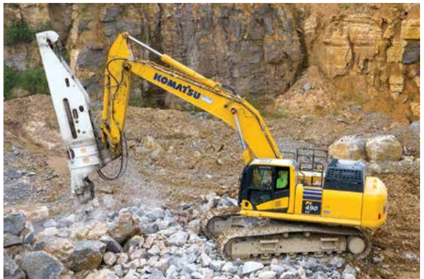
Using a Komatsu PC490LC excavator, an SEMO Quarry operator breaks boulders at the Cape Girardeau, Mo., site.
